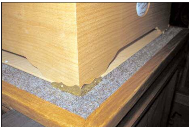
Figure 12. Brass corner secured through carpet to plywood. Figure 13. All brass corners attached to frame assembly. Figure 14. Brass corners hold organ in place.
