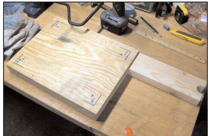
Figure 6 (below). Plywood cap atop the frame.
