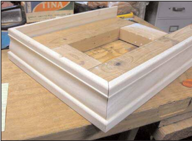
Figure 7. Adding trim molding to the frame.
